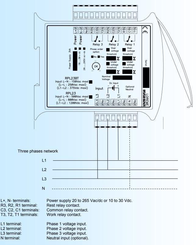
For a single phase alternative (AC) voltage, use inputs L1 and N. For a continuous voltage (DC), use inputs L1 and L2 (Dc input).
